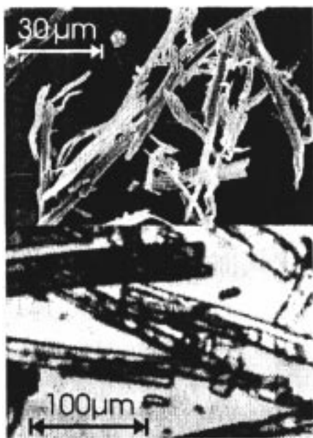
Figure 7. SEM micrographs of crystals of the A modification of Abecarnil obtained via an unseeded cooling crystallization from methanol (top) and photomicrograph of crystals of the A modification obtained via the seeded cooling crystallization (bottom). Note the differences in the scale bars.
